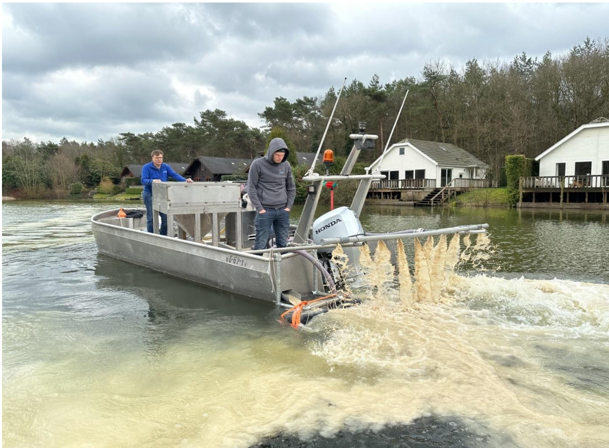
Figure 38: A Phoslock application showing the cloud of precipitant and the specialized equipment commonly used (Photo credit: Derek Johnson).
